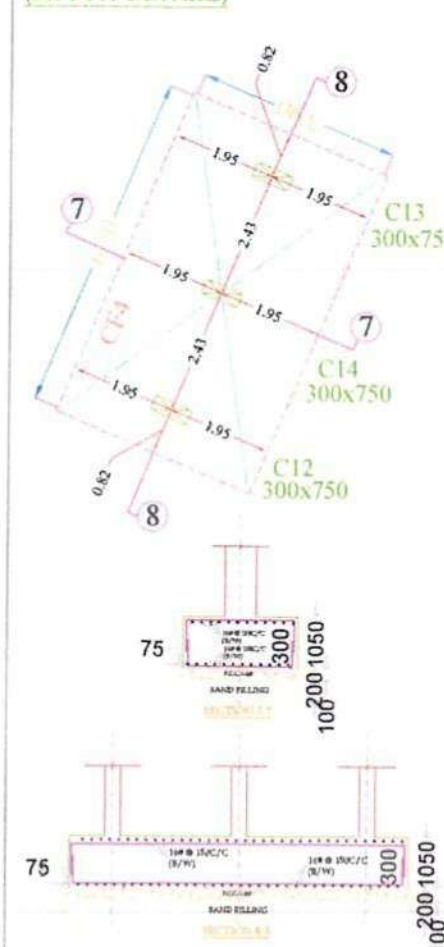
COMBINED FOOTING CF3- (6500x3900) (LIFT PIT DETAILS)
